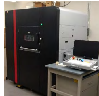
High-temperature SLS capabilities: Prodways HT2000 at Virginia Tech (left) and EOS-NA P400 at KCNSC (right)
