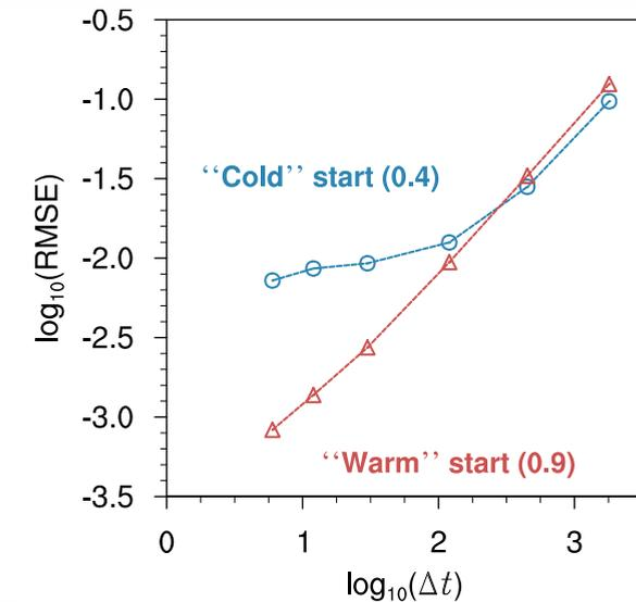
(a) Solution error and self-convergence and (b)-(c) time evolution of cloud fraction in single-column simulations with CLUBB (case: DYCOMS RF02)
