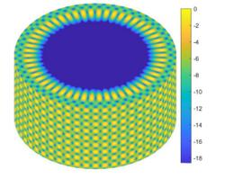
TM<sub>10,8,2</sub> mode of a RF cavity
