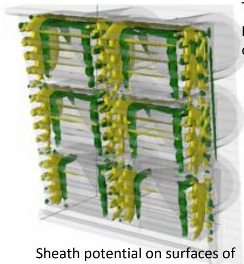
Sheath potential on surfaces of ITER ICRF antenna module
