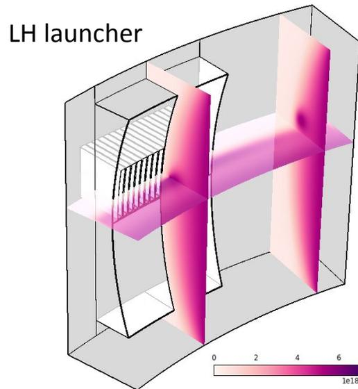
Field aligned density modulation placed in front of LH launcher. The modulation was computed by solving the diffusion from particle source in front of the launcher.
