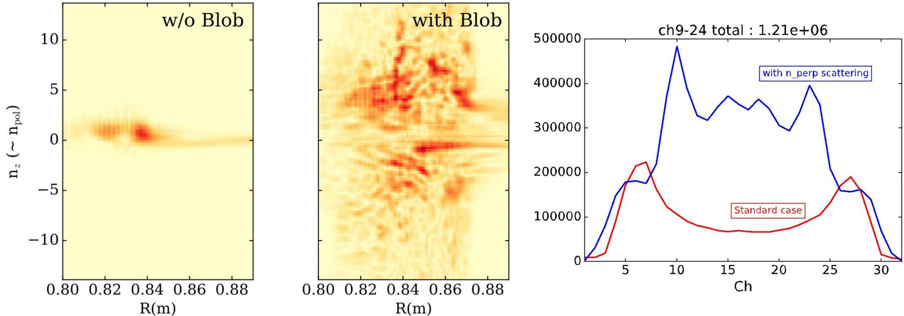
Perpendicular wavenumber spectrum is broadened with the blob.
