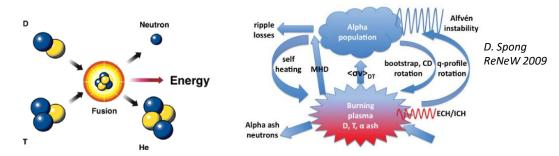
In a burning or self-heated plasma, the fusion process itself provides the dominant heating source for sustaining the plasma temperature
