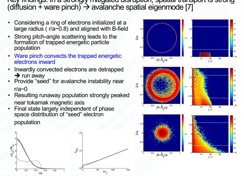
Runaway electron simulations are performed by LAPS-RFP code: relativistic Boltzmann-Fokker-Planck for both small- and large-angle collisions, radiation damping, quasilinear diffusion for wave-particle interaction, bounce-average; has both continuum and particle methods
