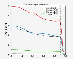
Core-pedestal Impurity profile prediction (OMFIT-based fast workflow)
