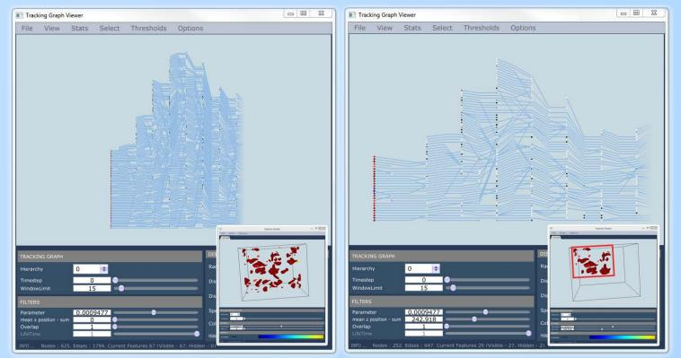
TALASS enables interactive threshold selection an features. computes and adjusts the tracking graph on-the-fly and provides the ability to select features based on size or spatial location.
