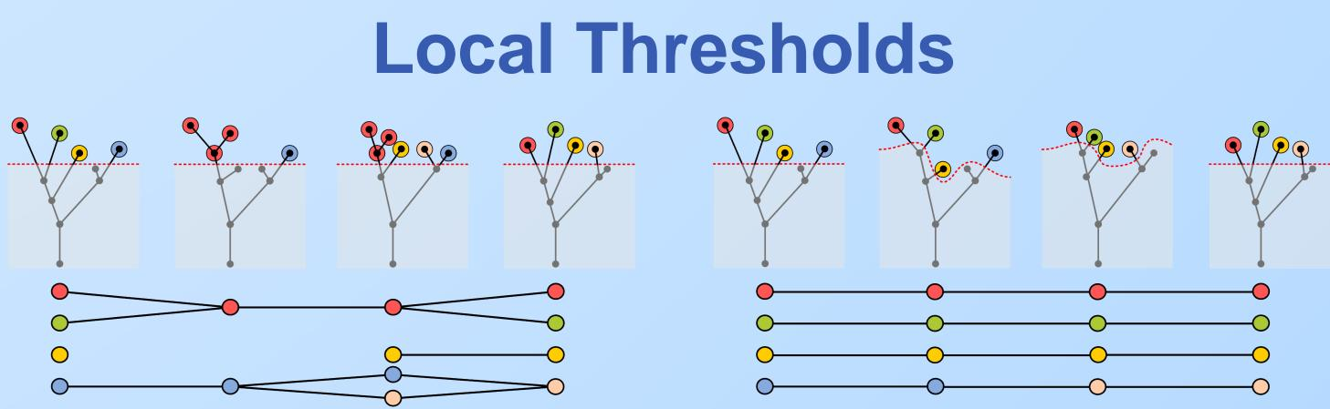
Using fixed thresholds creates spurious events in the tracking graph (left) due to instabilities in the threshold and artifacts of the linear interpolation in time. Given a small error tolerance in the threshold allows to locally adapt the feature definition to create a cleaner, more intuitive tracking graph.
