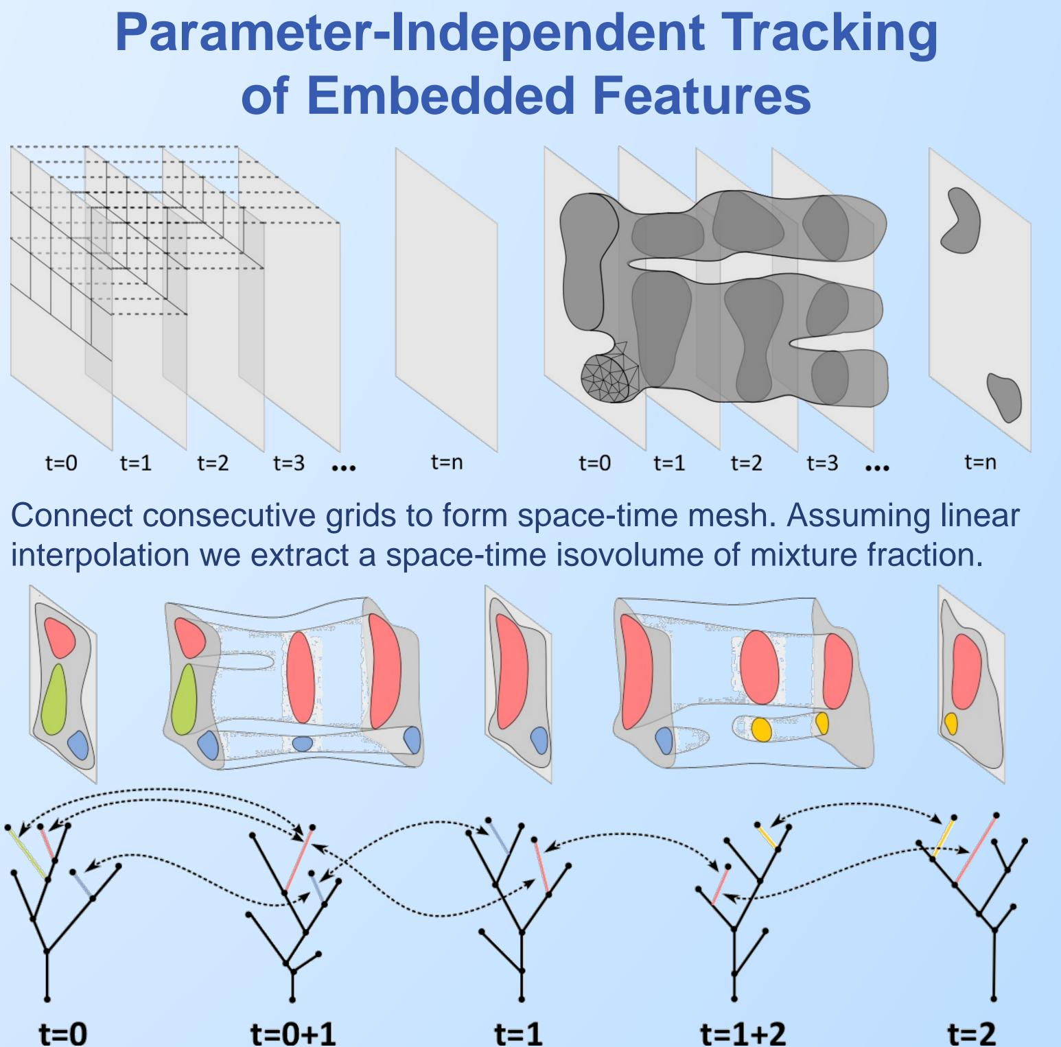
Computing merge trees within each time step provides parameterindependent feature detection. Merge trees of the combined spacetime mesh of consecutive time steps enable simple overlap tracking.
