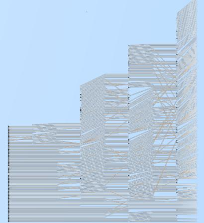
Tracking graph of the first time steps of the extinction regions in a di-methyl ether flame. (Left) Original graph; (Middle) Sub-selection by feature size. (Right) Modified graph using adaptive threshold to produce cleaner tracks, easier to understand and analyze.
