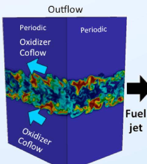
Problem: Define the flame as mixture fraction isosurface and analyze how the actively burning portions of the flame (red) develop extinction holes (dark blue). The goal is to track holes over time to understand how they form, grow and ultimately heal.
