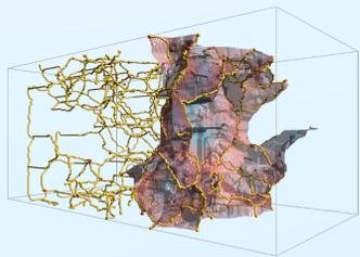
Screenshot from the **MSCEER** tool, showing interface surface of an impact into a porous medium as represented by steepest ascending surfaces between outside and inside. Skeleton of porous structure represented as steepest ascending lines in the density field.
