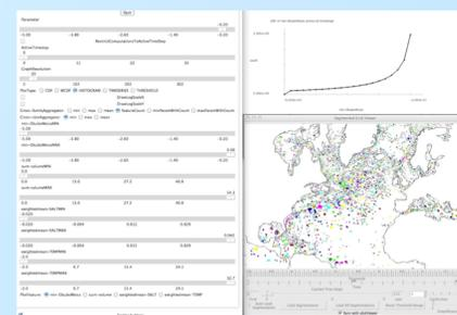
Screen capture of the TALASS tool showing interactively extracted eddies from an ocean simulation. (Left) Subselection interface allowing to filter features by attributes. (Top right) Global distribution of Okubo-Weiss parameter for all features. (Bottom right) Three-dimensional Feature display
