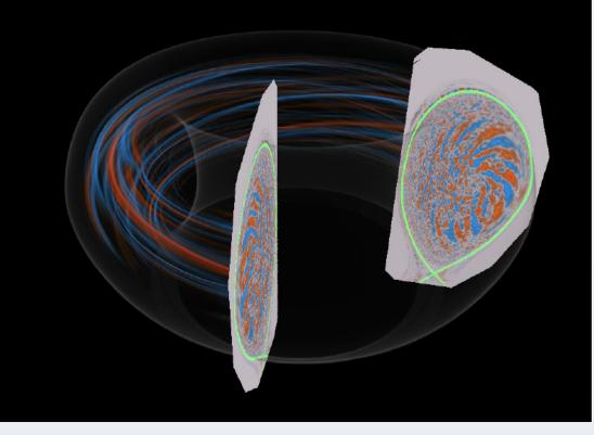
Large scale turbulence in the whole volume simulation in DIII-D geometry
