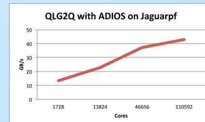
For the QLC2Q quantum turbulence code, ADIOS has enabled runs of up to 110K processes writing at upwards of 40 GB/sec (left).
