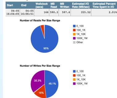
Example of NERSC web portal data available to Hopper end-users once a job has completed. Darshan data is used to automatically produce a graphical summary indicating the access size distribution, the amount of data accessed, estimated performance, and percentage of time spent performing I/O. Users can use this data as a starting point to evaluate I/O performance and validate application behavior.
