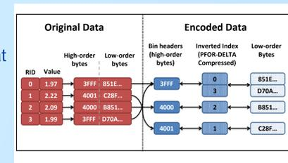
DIRAQ produces indexes that are up to 6x smaller than those of start-of-the-art indexing techniques, with the defragmented indexes resulting in an order of magnitude improvement in query performance. Overall, the integrated data compression and indexing method in DIRAQ results in a storage footprint of only 55-90% of the raw data size (a net reduction, including the added query index).
