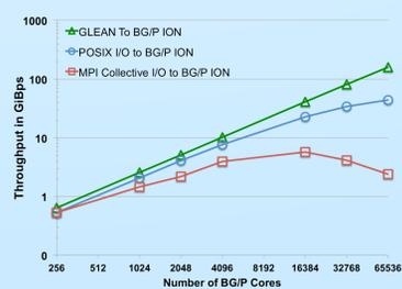
Strong scaling performance for 1GiB data movement off ALCF Intrepid Blue Gene/P compute nodes. GLEAN provides 30-fold improvement over POSIX I/O at scale. Strong scaling is critical as we move towards systems with increased core counts.
