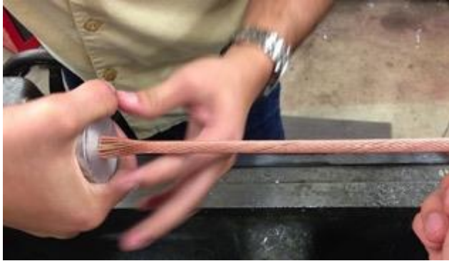
cabling wires onto perforated spring tube
