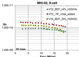
VT2; post Bipolar EP with 4% of H<sub>2</sub>SO<sub>4</sub>, but NO 120C bake
