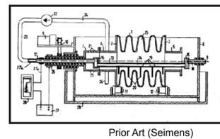
"Method for the electrolytic polishing of the inside surface hollow niobium bodies" U.S. Patent No. 4,014,765 issued March 29, 1977.
