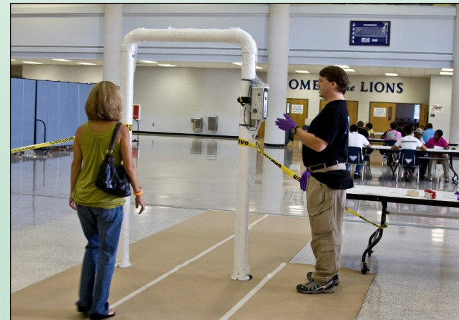
Image 1: Full-body contamination screening with a portal monitor
