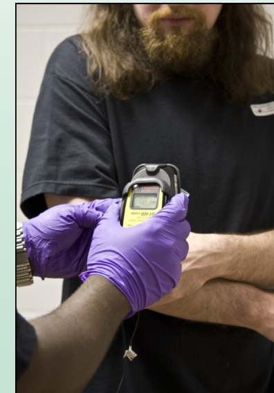
Image 2: High Contamination Screening with a Count Rate Meter
