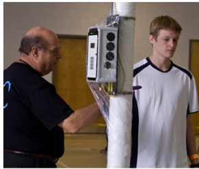
A survivor walks through a portal monitor. Portal monitors are another way to detect contamination.
