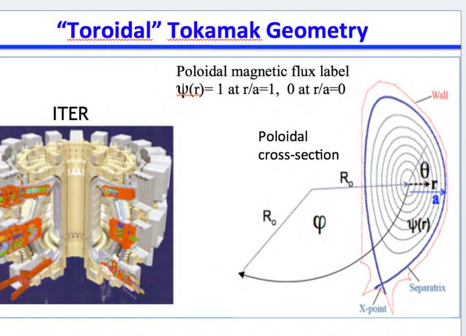
Torus, not a straight cylinder: physics becomes more complicated through the magnetic inhomogeneity and the toroidal mode coupling.
