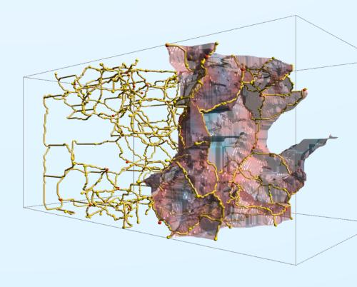
Screenshot from the **MSCEER** tool, showing interface surface of an impact into a porous medium as represented by steepest ascending surfaces between outside and inside. Skeleton of porous structure represented as steepest ascending lines in the density field.
