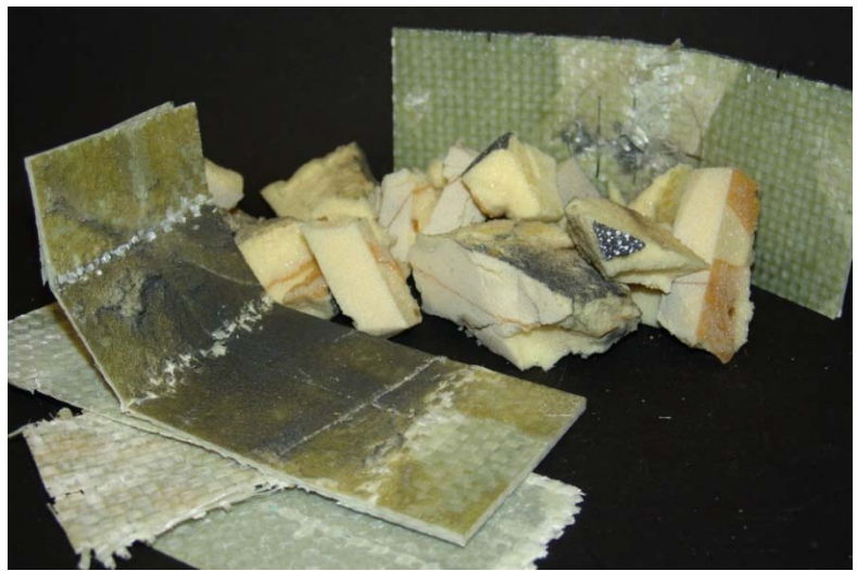
Specimen with Low Velocity Impact Damage
