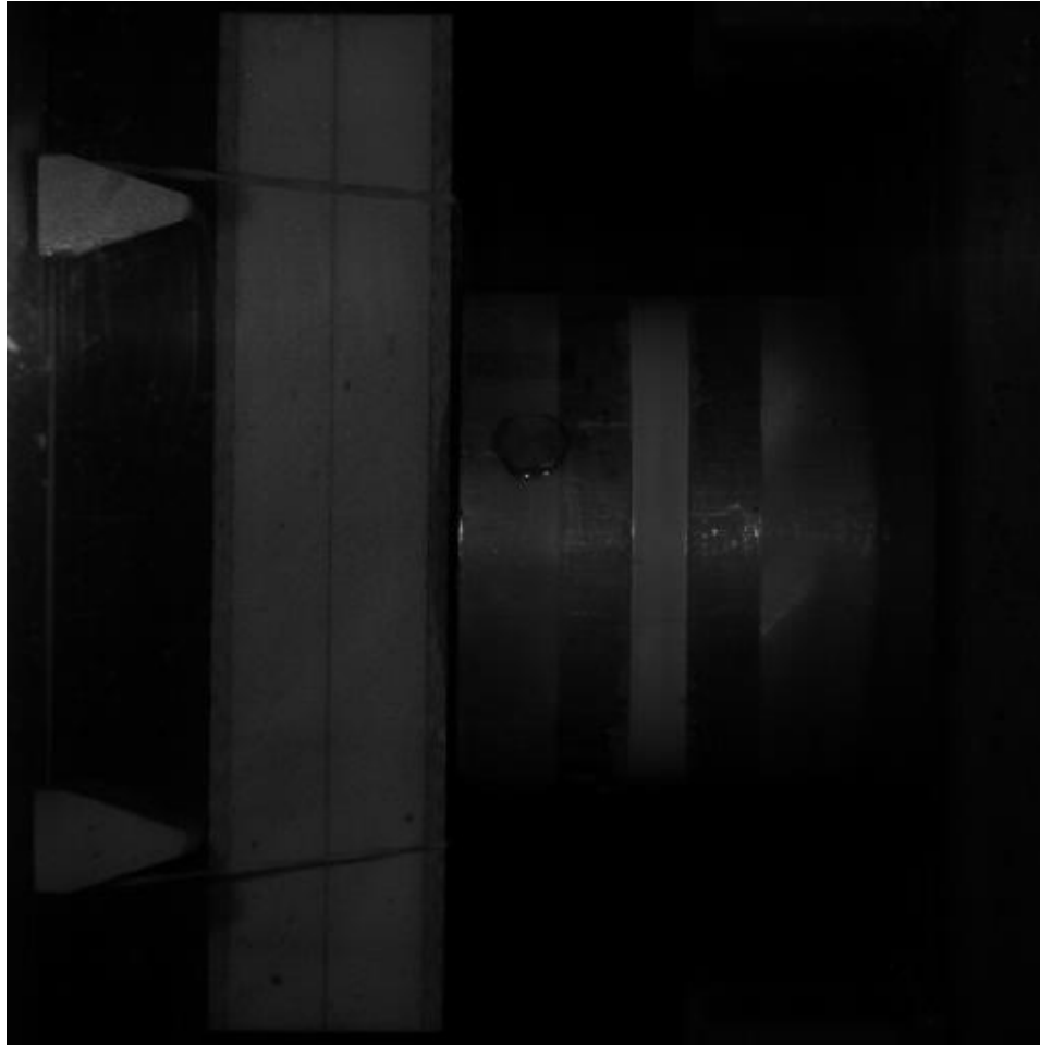
E-Glass Vinyl Ester Composite — Corecell Foam Sandwich under blast load
